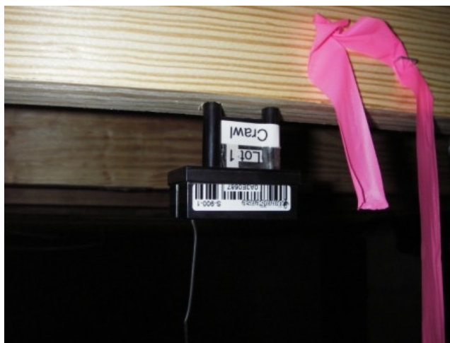
Figure 22. Crawl space OmniSense sensor mounted on floor framing.
